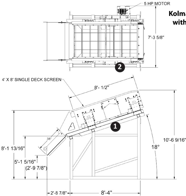
**Kolman 4'x8' Single Deck Screen with 18 degree Inclined Stand**
