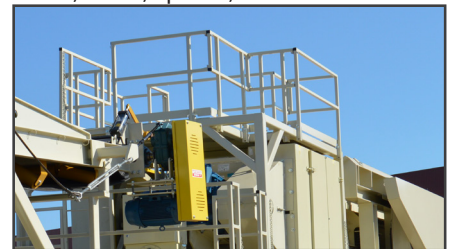
Upper and Lower Platforms Double Handrails and Kickplates
