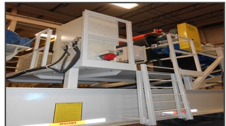
Access Platform with Double Handrails and Access Ladder
