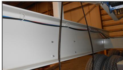
Heavy Duty Wide Flange Beam Chassis
