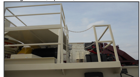
Diamond Plate Platforms Double 2" Handrails and Kickplates
