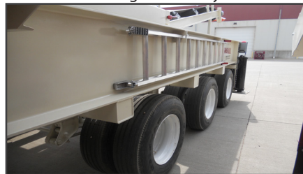
Wide Flange Beam Chassis
