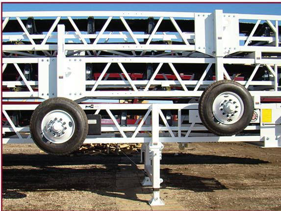
Offset axles for easy unstacking and stacking
