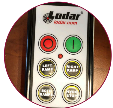
Wireless Remote Control Easily cycle your ramps from the comfort of your cab.
