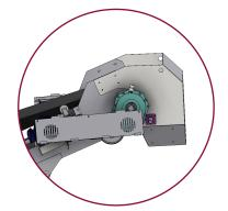
**Discharge Hood**with AR liners to feed 36"
