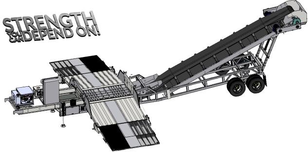
Masaba's Low Profile Truck Unloader is an easy, portable option to keep unloading simple. Our truck unloaders are built with a heavy duty steel tubing frame. The self-deploying hydraulic ramps allow for easy placement in your operation and remove the need for earthen ramps. The 48" discharge conveyor comes with an AR lined discharge hood, perfect for feeding a stacker or other equipment in your spread.
