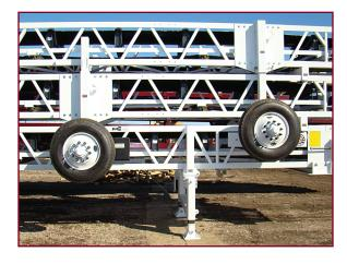
Offset axles for easy unstacking and stacking
