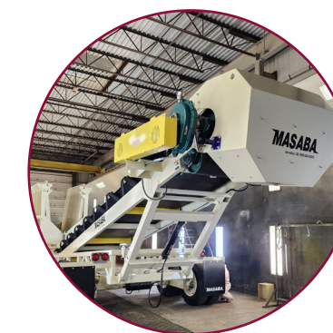
Discharge Hood With AR liners to feed 36" belt width or greater.
